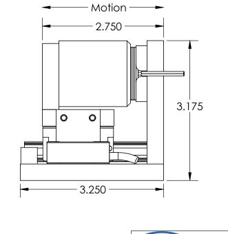
UNLESS SPECIFIED OTHERWISE: All dimensions are in inches Standard Tolerances are as follows XXX ±0.05 ANGLES ±1° XX ±0.10 FILLETS 0.10 X ±0.20 CORNERS 0.10 Remove All Burrs and Sharp Edges
