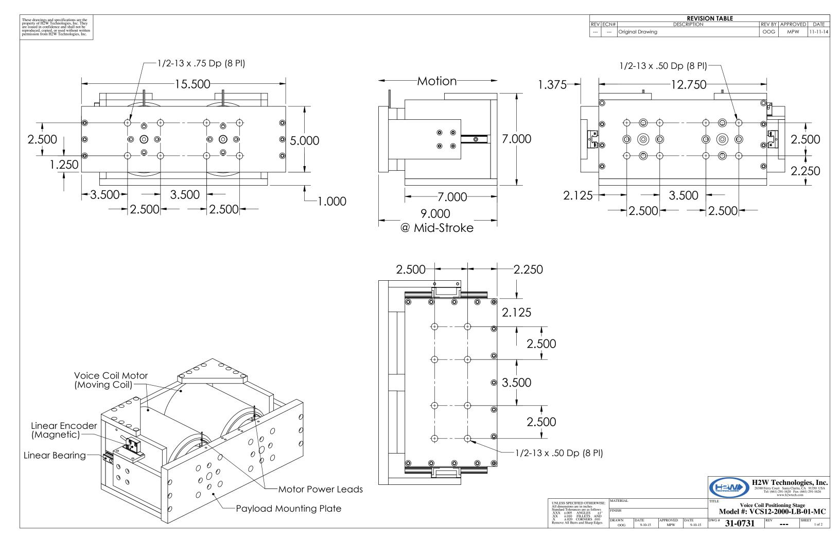
These drawings and specifications are the property of H2W Technologies, Inc. They are issued in confidence and shall not be reproduced, copied, or used without written permission from H2W Technologies, Inc.
